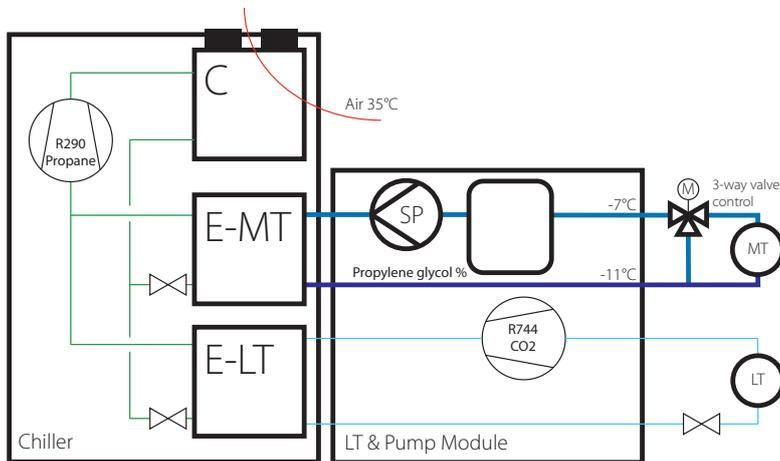
Medium temperature desks and storages (MT load) are cooled by propylene glycol solution (brine). Brine is pumped in the closed loop between MT load and Felzer AirGREEN brine liquid chiller with R290 (Propane) green refrigerant. MT load increases brine temperature from -11C to -7C and Chiller decreases it from -7C to -11C in the first evaporator (E-MT). And in the second evaporator (E-LT) the same unit condensates CO2 in subcritical low temperature cycle.
